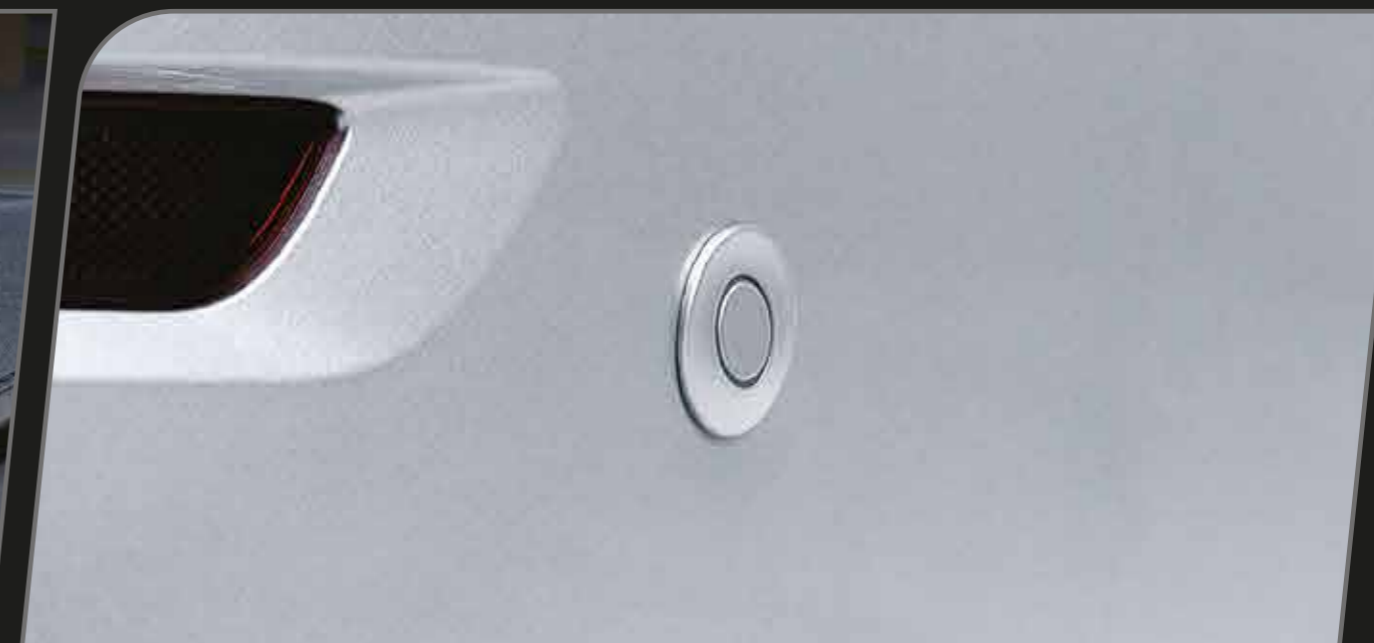
REAR PARKING SENSORS
