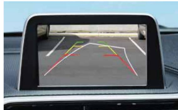
The dynamic reverse guidelines trace the vehicle's trajectory and assist in steering conveniently without colliding into obstacles.
