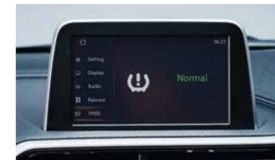
Pakistan's 1st sedan with Tire Pressure Monitoring System (TPMS) offers tire pressure on the driver's screen. The system provides alerts to the driver before the tire deflates to ensure safety of passengers.
